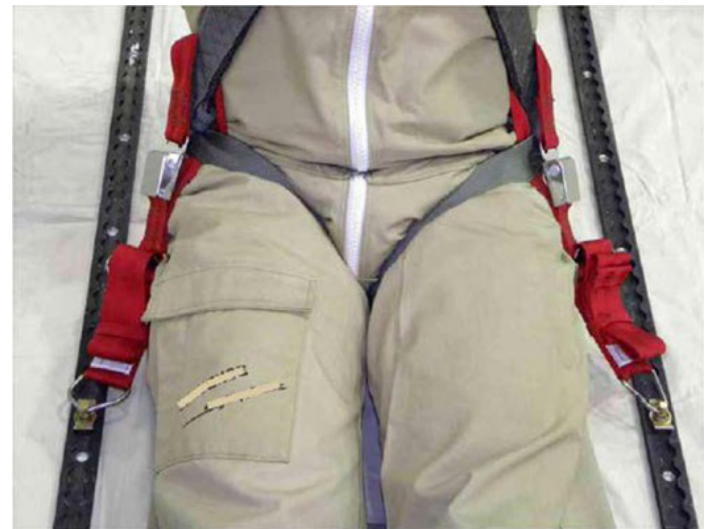
Figure 8. Dual Point, Dual Tether Restraint Configuration For Rear-Facing Floor Seats
